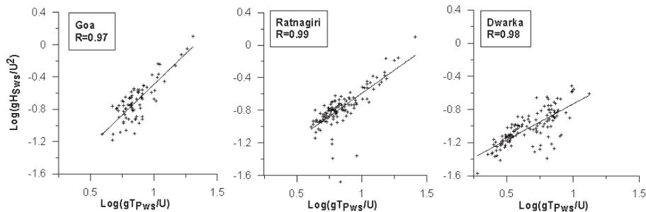
**Fig. 8.** Scatter between  $\log(gH_{\text{sws}}/U^2)$  and  $\log(gT_{\text{pws}}/U)$  at different locations along the west coast of India.
