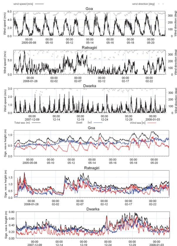
**Fig. 2.** Wind parameters (wind speed and direction) and significant wave height (total sea – black, swell – blue and wind sea – red) off Goa, Ratnagiri and Dwarka.
