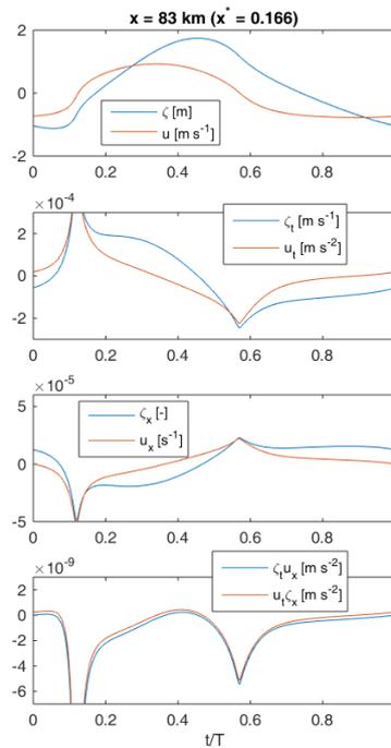
**Fig. 5.** Temporal variation of  $\zeta$  and  $u$  (first plot),  $\zeta_t$  and  $u_t$  (second plot),  $\zeta_x$  and  $u_x$  (third plot), and  $\zeta_t \ u_x$  and  $u_t \ \zeta_x$  (fourth plot) in  $x=83$  km.
