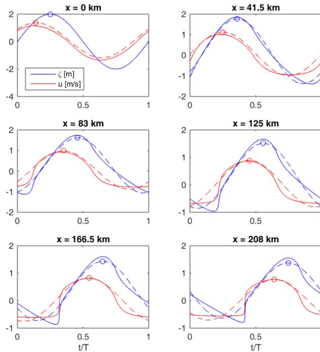
**Fig. 9.** Tidal waves and Fourier series truncated at the first harmonic. Circles indicate the maxima of the dominant tidal component, from which it is possible to detect the phase lag  $u-\zeta$ .
