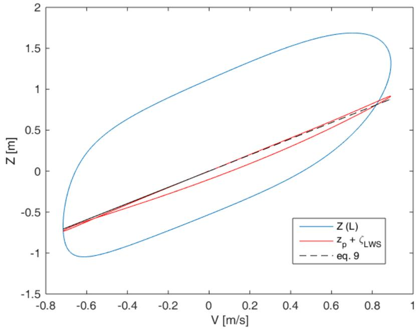
**Fig. 14.** Lagrangean water level against velocity  $V$ :  $Z$  is the actual value,  $z_p + \zeta_{LWS}$  is the transformed water level. Black dashed lines: equation (9).
