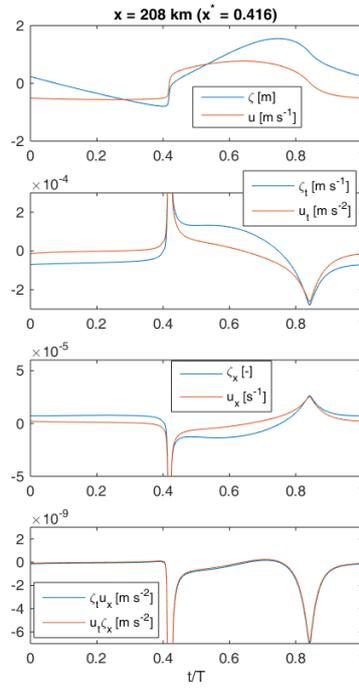
**Fig. 8.** Temporal variation of  $\zeta$  and  $u$  (first plot),  $\zeta_t$  and  $u_t$  (second plot),  $\zeta_x$  and  $u_x$  (third plot), and  $\zeta_t \ u_x$  and  $u_t \ \zeta_x$  (fourth plot) in  $x=208$  km.
