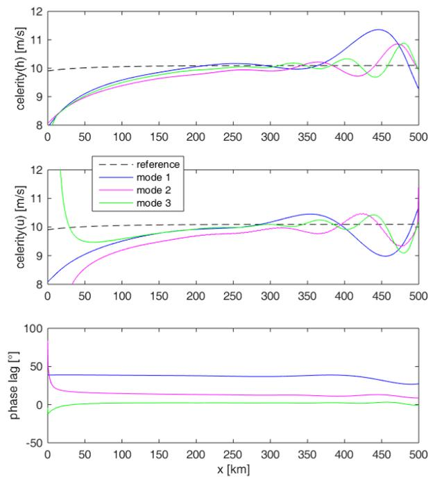
**Fig. 11.** Wave celerity for water level  $\zeta$ , for velocity  $u$ , phase lag  $u - \zeta$ . Colors refer to the first three modes; black dashed line to wave celerity in a frictionless prismatic channel.
