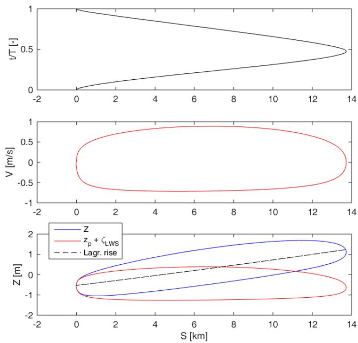
**Fig. 13.** Lagrangean displacement  $S$  in time (first plot) and ellipses  $V$ - $S$  (second plot) and  $Z$ - $S$  (third plot).
